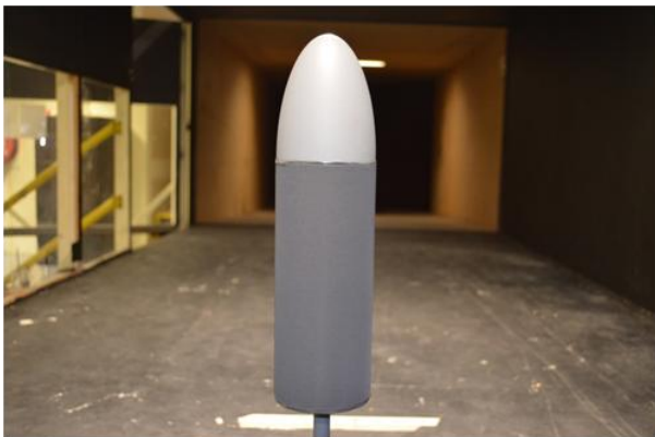
Fig. 3: Test cylinder fitted with fabric sample.
